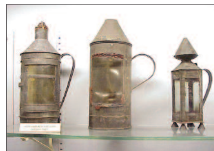
Figure 12. Royal Institution: Davy's early designs of the safety lamp utilized small holes to cool the gases emanated from oil lamps so that pockets of firedamp would not be ignited.
